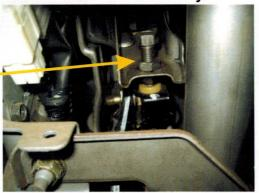
Replace the stop-bolt with the enclosed clutch switch.
