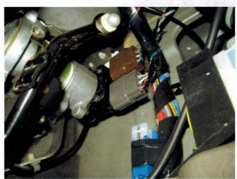
Connect the throttle pedal interface harness between the throttle pedal & the vehicles harness. (Connect all 3 pairs of connectors).
